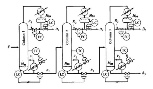
Q2. Flooded condensers and flooded reboilers are sometimes used on distillation columns. In the sketch below, a liquid level is held in the condenser, covering some of the tubes. Thus a variable amount of heat transfer area is available to condense the vapor. Column pressure can be controlled by changing the distillate (or reflux) draw-off rate. Write the equations describing the dynamics of the condenser.
